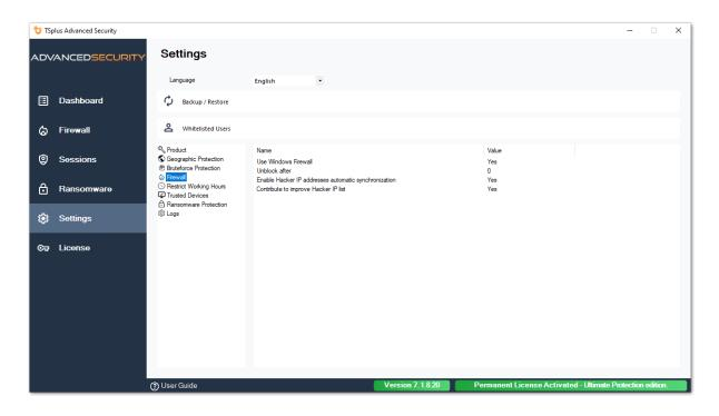
**Use Windows Firewall** In order to activate the built-in firewall, go to Settings > Advanced > Product > Use Windows Firewall and set the value to: No If Yes, then the offending IP addresses will be blocked using Windows Firewall. TSplus Advanced Security firewall will be used otherwise.
