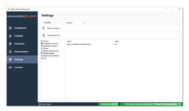
TSplus Advanced Security's Trusted Devices cannot resolve the client name if the connection is initiated from TSplus Remote Access' Web portal. Therefore, Trusted Devices will block any connections from Web Portal by default. Set this setting to "Yes" to allow connections from the Web portal. Please be aware that this action will diminish your server's security.
