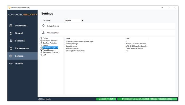
**Warning message schedule** You can configure in number of minutes before the user is automatically disconnected. By default, it is set to 5 minutes.
